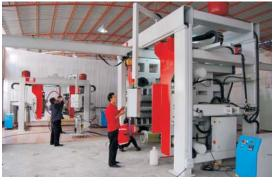
We present a unit for the production of hollow insulators. insulators ranging from 88 to 500 kV may be produced with this machine. Moreover, we can offer passable closing units with clamping surfaces between 1,000 x 750 mm - 3,000 x 1,600 mm. All our machines are supplied as turnkey units, including moulds for the various sizes requested, on a global basis.
